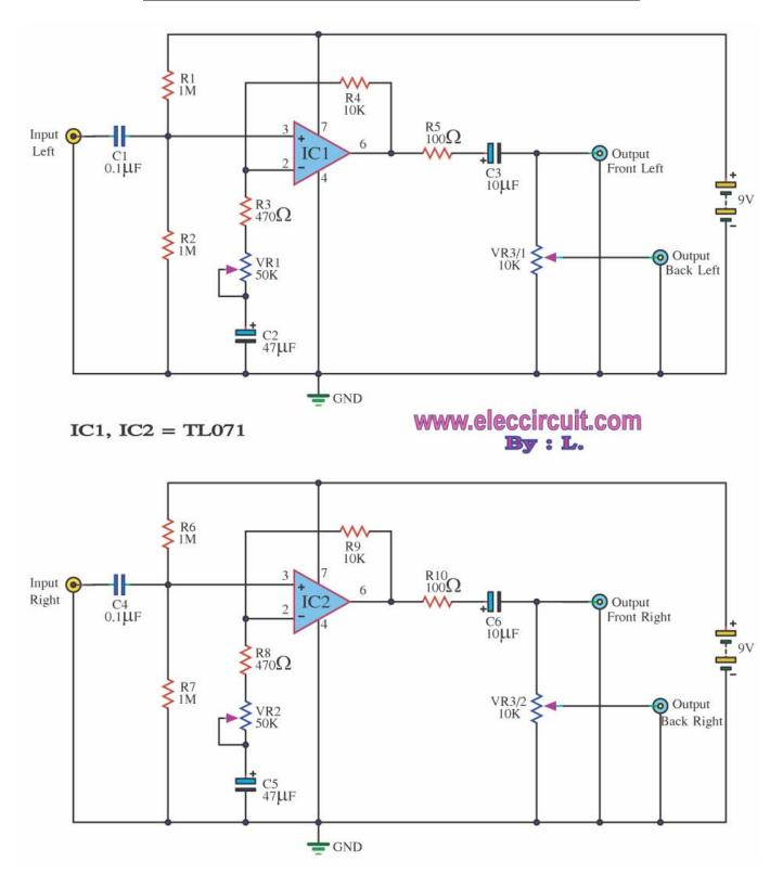
This circuit can be used on Car audio stereo systems that only have front speakers only a single page. The circuit will increase the number of speakers up to the other two to be connected to the back speakers pair.
